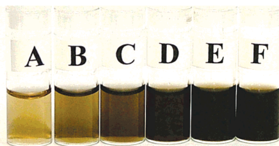
Figure 1. Photographs of SWNT dispersions of various concentrations in deionized water: (A) 0.05, (B) 0.1, (C) 0.2, (D) 0.3, (E) 0.5, and (F) 2 mg/mL.
